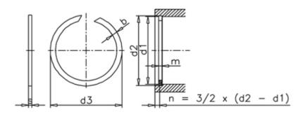
$\begin{array}{lll} b & = 3.40 \\ d1 & = 105 \\ d2 & = 107.3 \\ d3 & = 108.3 \\ Description = SB 105 \\ FN kN & = 63.80 \\ FR kN & = 51.80 \\ m min & = 2.7 \\ \end{array}$
